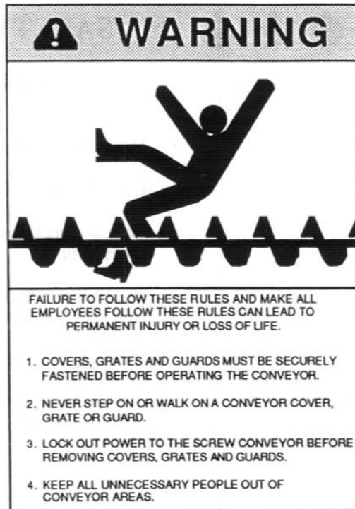
Figure 2-2 Warning Label Above The Ice Discharge
