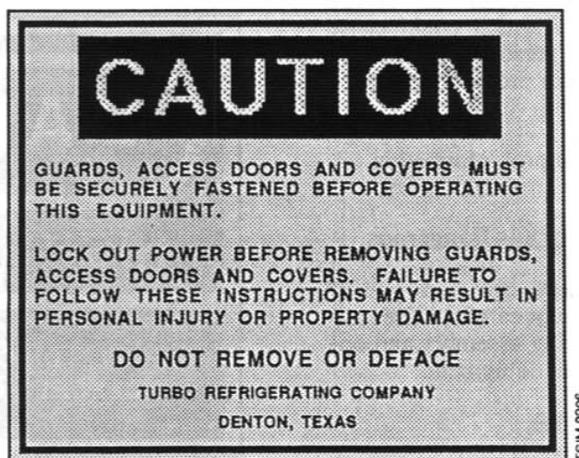
Figure 2-3 Warning Label On The Access Panels And Above The Ice Discharge
