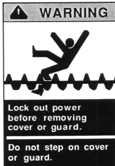
Figure 2-4 Typical Warning Labels On Screw Conveyor Covers And/Or Belt Pulley Guards
